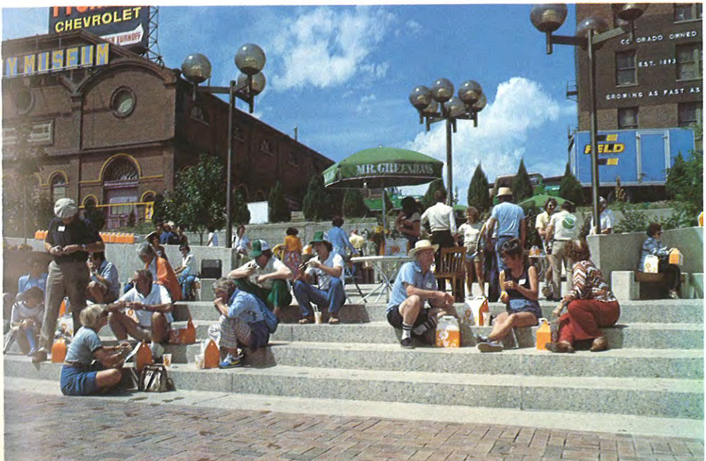
The plaza after construction, with the Forney Museum and the H. H. Post buildings in the background. The brick landings and terrazo steps have been inundated a few days each spring since 1975 with no damage.
